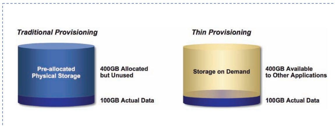
Figure 1) NetApp thin provisioning (just-in-time storage).
